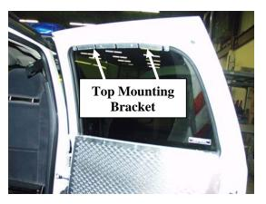
• With top mounting bracket for hinging window guard attached, hinge window up and mark placement for top mounting bracket.
